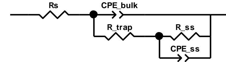
$R_{\text{trap}}$ : the resistance associated with the charge recombination at the surface states
